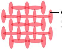
Simulated light dispersal of laser diodes closely spaced. Overlapping light spots provide more even coverage.
